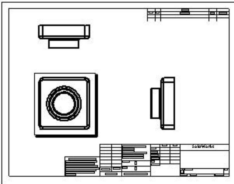
*Drawing views are containers. Generally the contents are views of models. When you sketch in a drawing, or insert annotations or blocks, the entities belong to the active drawing view or drawing sheet.*
