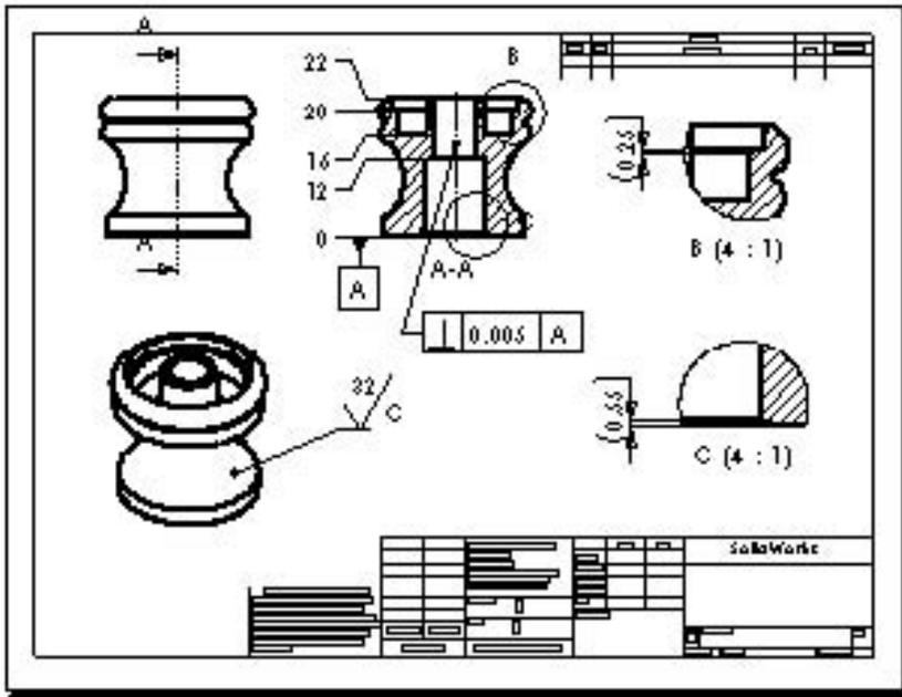
Section views are aligned automatically in the direction of the cut. Detail views are not aligned.
