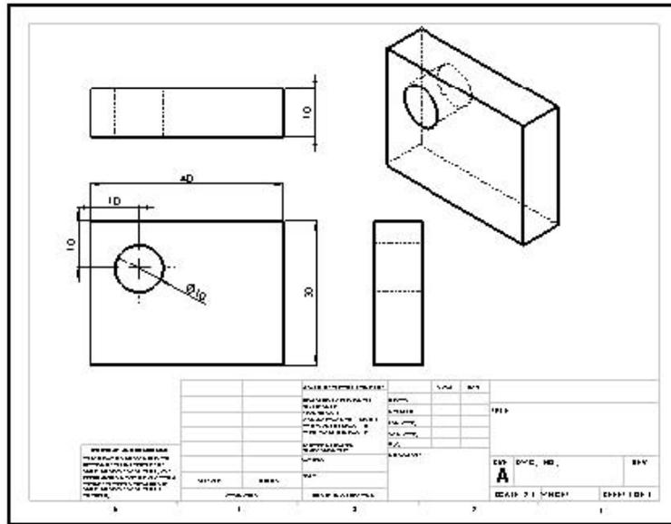
Model part Drawing with several views and dimensions inserted
