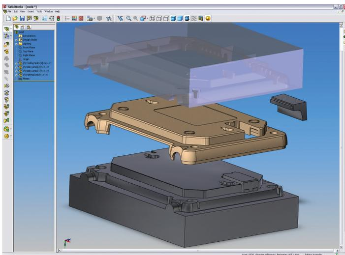
SolidWorks software provides tools that allow you to easily move from a part design to generate all the core and cavity geometry necessary for machining.
