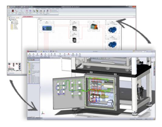
With SOLIDWORKS Electrical Professional, single-line and multi-line schematic tools, including an integrated library of thousands of symbols and parts, enable quick planning of your embedded electrical system.
