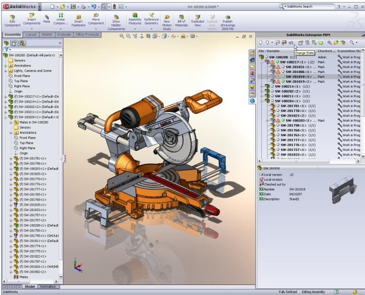
SolidWorks Enterprise PDM facilitates workflow management, revision control, design reuse, and cost control for equipment or process designs.
